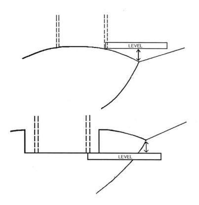
Reference the aft landing spot with the edge of a level over to the corner of the boat and measure the difference. Measure both sides of the boat and average the two.
