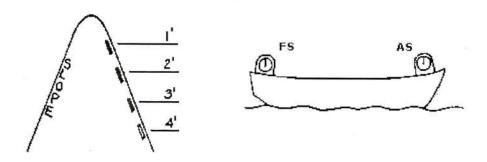
**ROLL** is the camber of the deck. It is measured on a line <u>perpendicular to the edge of the deck</u>. There are two kinds of roll.
