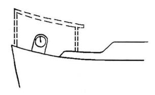
IMPORTANT: Measure the angle of the shear line with the angle gauge as shown. If there is a combing under the forward landing spot, provide the measurement of the height from the top of the deck to the top of the combing.
