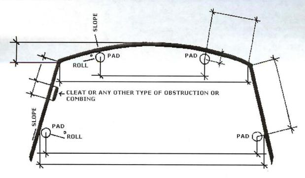
Measure the slope and roll angles at one-foot intervals as far forward as the stern rail will cover.
